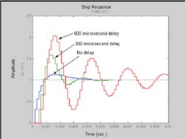
Figure 5. In this plot of proportional-integral (PI) controller step response with varying delays, notice how increasing the delay degrades performance.
