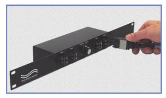
fastened with steel hardware for rugged durability. The Model 9163 enclosure is an ultra slim rackmount package, 1U high and 19 inches wide to mount into a standard 19 inch equipment rack frame or cabinet.
