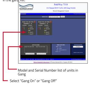
Figure 2: Multiple Model 7318's displayed in the GUI.
