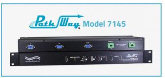
The unit monitors data activity on both ports "A" and "B". If activity on the connected port is lost for 2 seconds, and if the other port has established valid activity, the unit automatically switches to the port with valid activity. As long as there is activity on the present port, the unit will maintain the connection with that port. If neither port has activity, it will stay connected to the present port.
