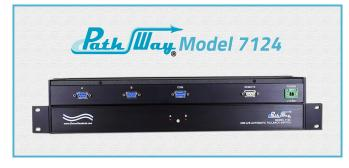
The Model 7124 will maintain its connection to the Port "B" until data activity is detected on the Port "A", at which time the unit will automatically return to the "A" position. If no data is present on either the Port "A" or on Port "B", the unit will stay in the "B" position and continue to monitor for data. The user can override automatic fallback operation from the front panel or from the Remote Port and force the unit to operate as an A/B switch.
