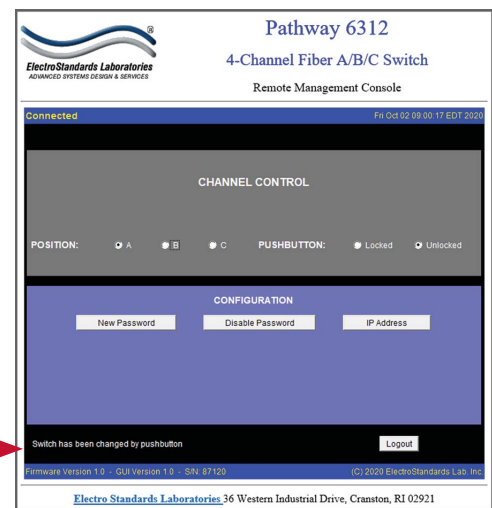
Figure 3: Change made via the front panel pushbutton. Alert shown in the Graphical User Interface.
