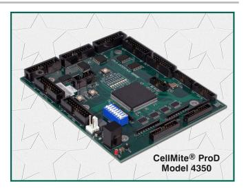
The CPLD interface board has 15 single-ended PWM input signals, 16 differential PWM output signals, 4 differential Brake output signals and a differential Inverter Enable output signal. It also has an 8-bit parallel LCD interface, 32-bit General Purpose I/O, 8 position DIP switch, 2 user pushbutton switches, a reset pushbutton switch and a 10MHz oscillator. For debug and test purposes the board has a 16-bit test port and 8 user LED indicators.
