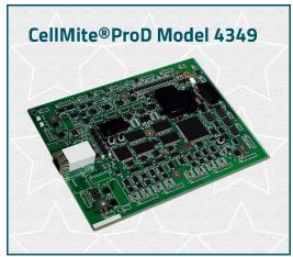
can be used to buffer transient event data. The CellMite® ProD features a wide input voltage range of 19VDC-36VDC, along with 3kVDC isolation. The CellMite® ProD is designed for ruggedized applications and is designed to operate from -40C to +85C.
