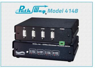
*both* destination devices, COM1 and COM2. Likewise, if the RTS signal is lost from the device connected to the D2, the Model 4148 automatically broadcasts the data from the D1 device to *both* the devices COM1 and COM2. One of the status LED's will be lit steady ON to reflect the connectivity status and signify that the unit is in Automatic Operation.
