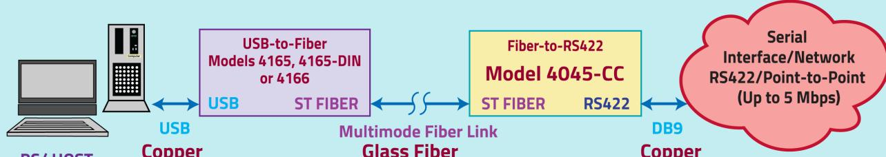
Isolated PC/HOST USB to RS422 communications serial interface/network.
