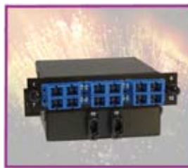
Model 6006 One 12-Fiber MTP/MPO input breaks out to 12 SC outputs (12 Simplex or 6 Duplex)
