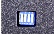
Figure 3: Dipswitch is located on the bottom panel of the unit.
