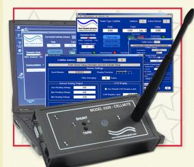
**CellMite** Model 4329 - Wireless DSC features a nonvolatile memory for parameter and calibration storage, the ability to select between 3 transducers, multi-point and mV/V calibration, remote sense excitation, and a 24-bit internal resolution with 16-bit analog output.
